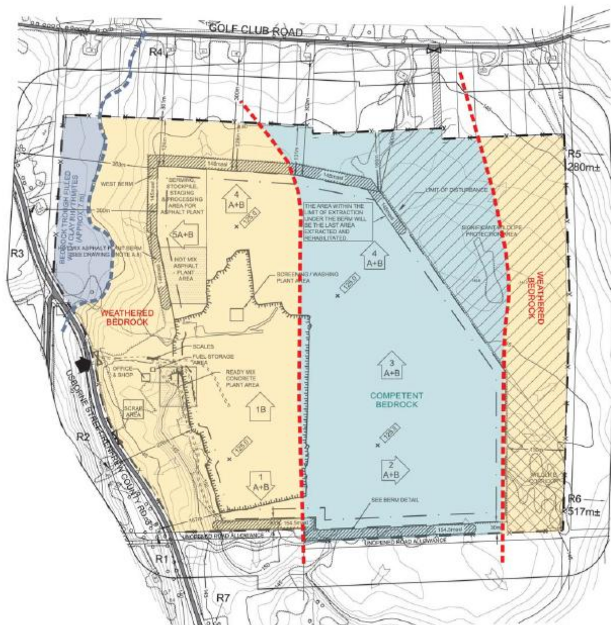
Figure 9 – Areas of Weathered Bedrock and Competent Bedrock
