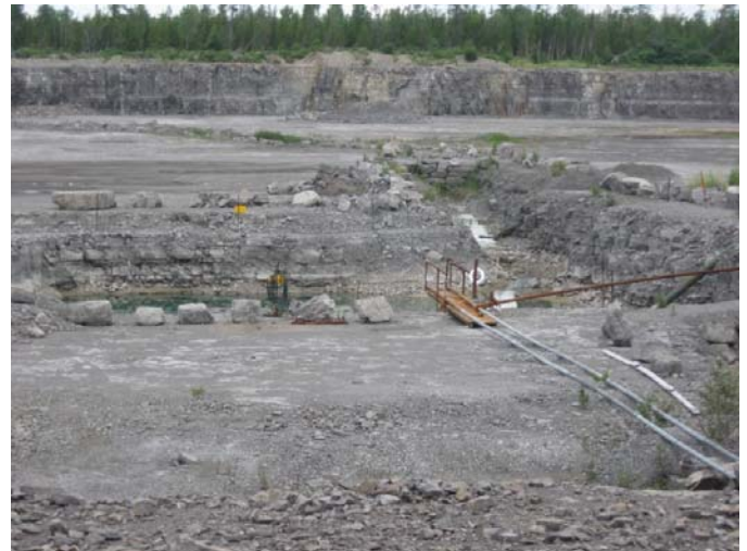
Photo 18: July 22, 2009; Sump level is significantly lowered and floor ditch has no flow
