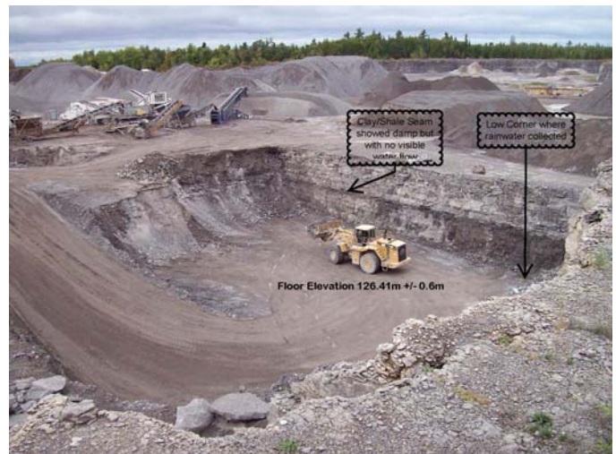
Photo 24: Annotated Photo taken September 3, 2009 as last of blasted rock removed from lower lift cut (Miller photo)
