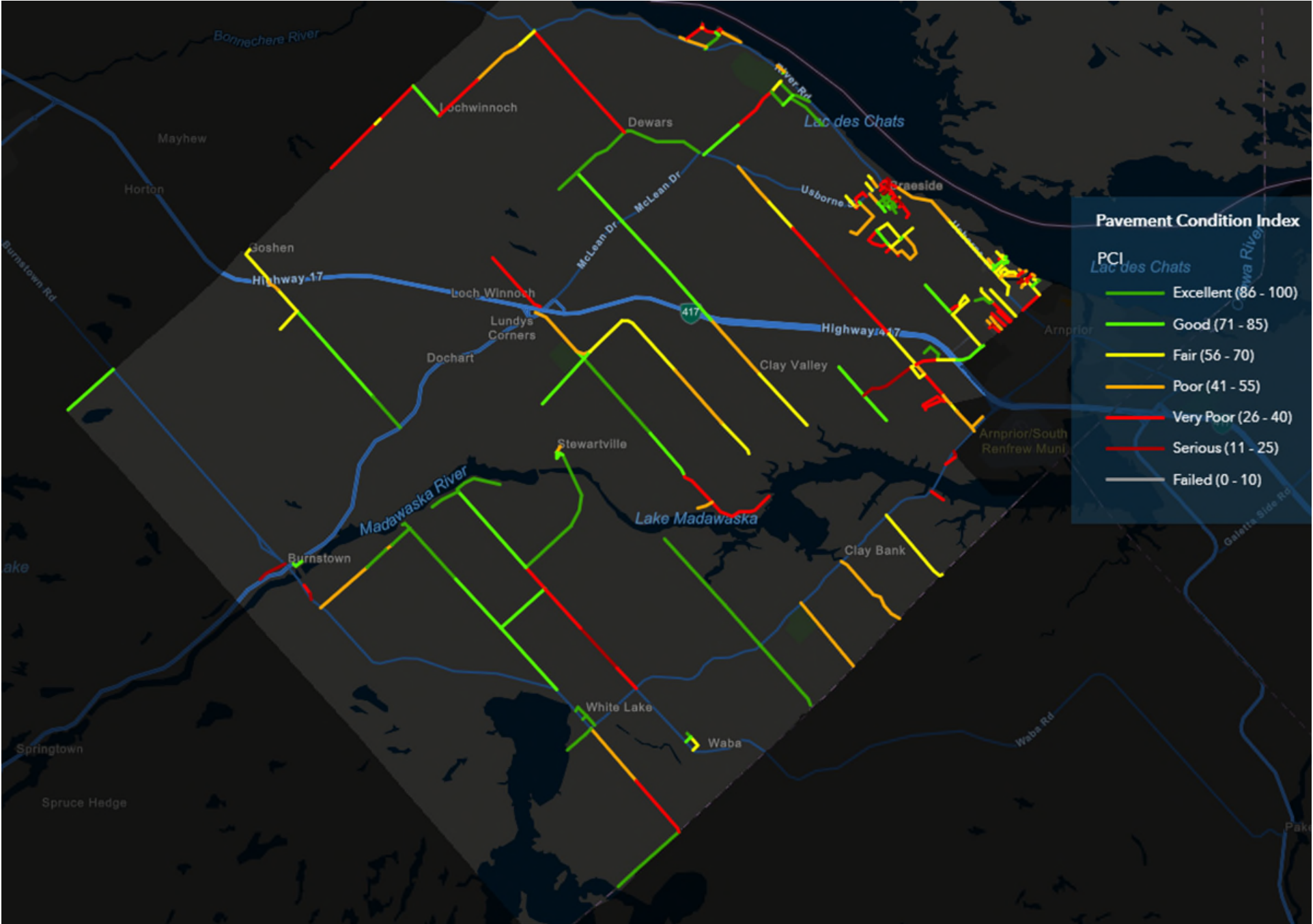
Township of McNab/Braeside – Paved Road Network (Pavement Condition) (As of end of 2024)
